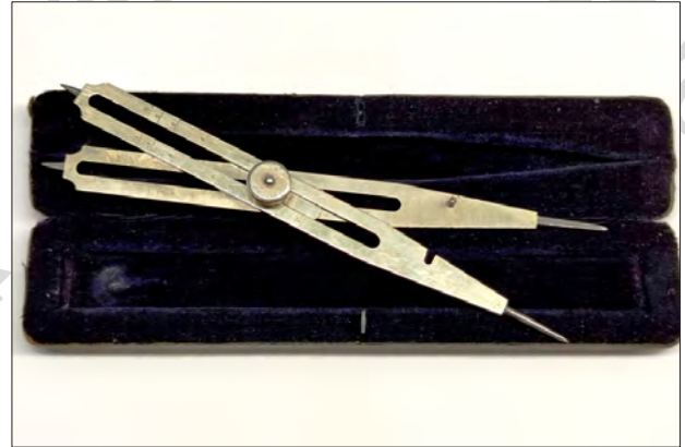
Proportional dividers made of white bronze from the patternmaking department of the former Lingel shoe factory in Erfurt.
